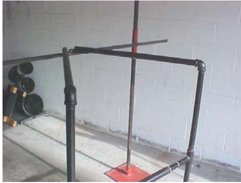
This is a picture of my homemade adjustable “V” Dipping Bars. I can adjust the height and width as well as the angle.
